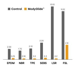
Coefficient of friction for various elastomers before and after ModyGlide™. Testing conducted per ASTM D1894-14.
