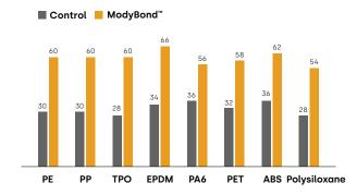
Sample surface energy enhancements (dyne/cm) with Inhance Technologies ModyBond™. Testing conducted per ASTM D2578-84.
